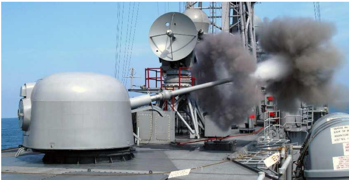
76 mm (3") Mark 75 aboard USS Curtiss FFG-38 in July 2003. Detail from US Navy Photograph No. 030718-N-4178C-002
